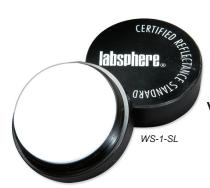
The WS-1-SL is a diffuse reflectance standard from Labsphere and is made from their patented diffuse reflectance material, Spectralon. Spectralon is hydrophobic and is thermally stable to 350 °C. The durable material provides highly accurate, reproducible data. Unlike all the other PTFE-based standards on this page, the WS-1-SL often can be smoothed, flattened and cleaned if nicked or soiled.
